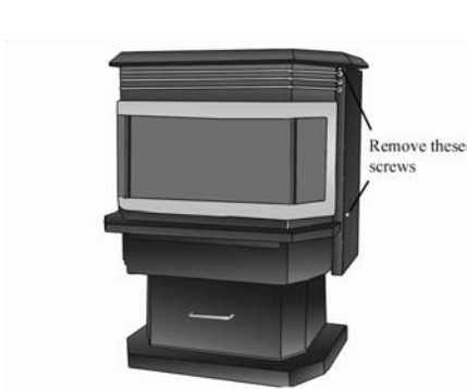
Figure 18. Holes for screws on the right side panel
