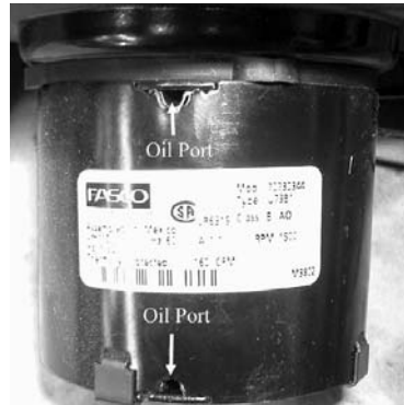
Figure 19. Oil ports on a circulation fan
