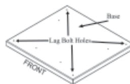
Figure 16C KSH Anchor Holes
