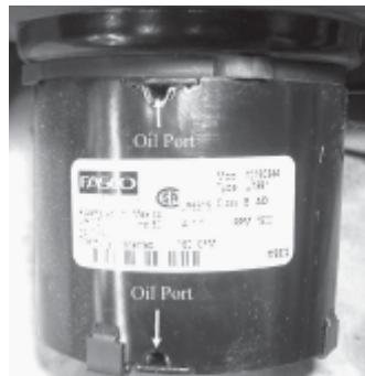
Figure 24. Oil ports on a circulation fan
